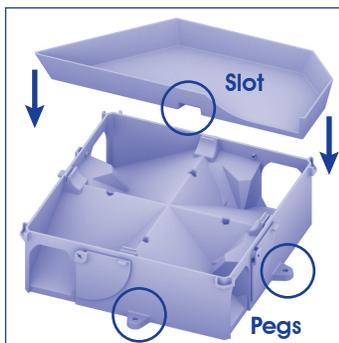
1. Attach a tray to the base by joining its slot onto the corresponding peg.
