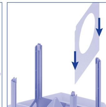
6. Slide a window into the slots of the window holders, as shown.
