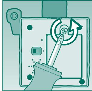
Turn the base over and, using a cross head screwdriver, turn the battery compartment screw anti-clockwise. Remove the battery compartment cover.
