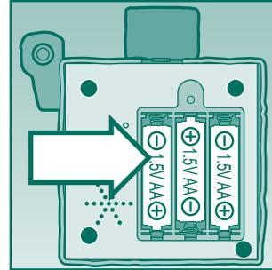
Insert 3 AA/LR06 batteries with the polarity as shown. Replace the battery compartment cover and tighten the screw gently.
